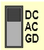
In the GND position, the input of the Y-amplifier is connected to 0 V. This allows you to check the position of 0 V on the oscilloscope screen.
