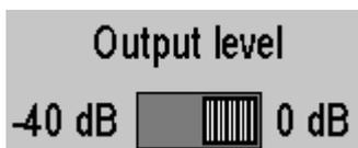
This gives an output signal with a peak amplitude which can be easily adjusted up to several volts. In the -40 dB position, the amplitude of the output signal is reduced to a few millivolts. Such small signals are used for testing amplifier circuits.
